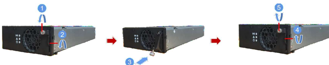
Figure 1-1 Installing a solar module
